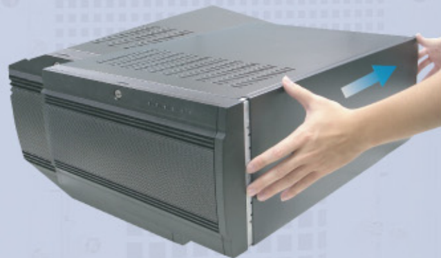
To remove top cover and bottom cover of chassis
