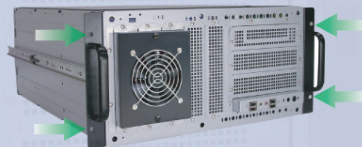
Screw in rack bracket and handles This is the illustration for model YY-W2XX Type B. Please refer exact spec. of each Type.
