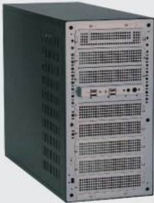
Type A: 8*5.25" drive bays+2xHDD Bracket
