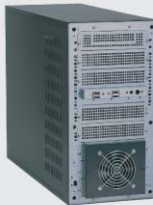
Type B: 5*5.25"+7*3.5"HDD drive bays
